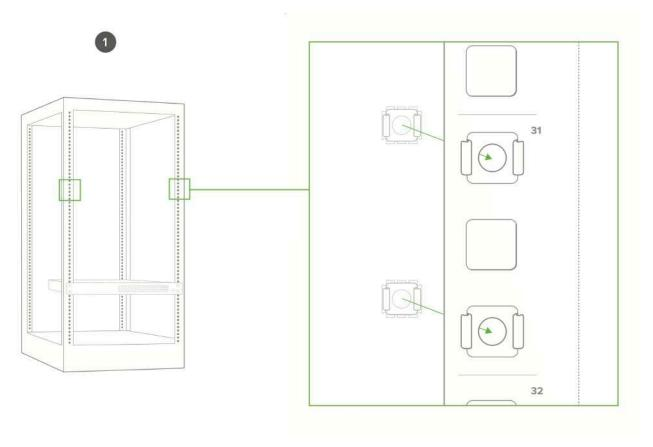
2. Attach the switch face plate to the cage nuts on the rack.
