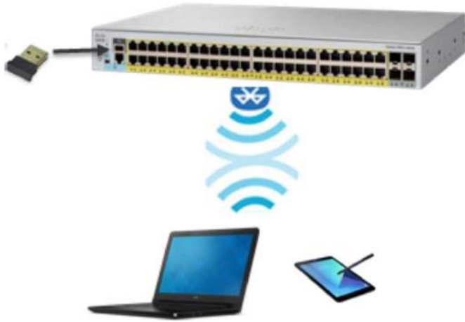
Figure 4. Over-the-air switch access using Bluetooth
