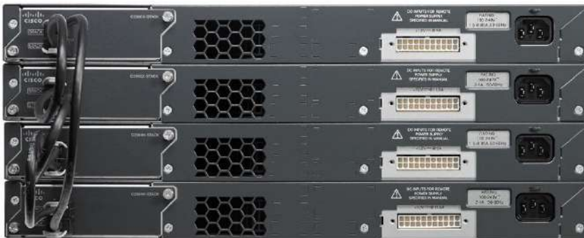
Figure 5. Cisco FlexStack-Plus switch stack
